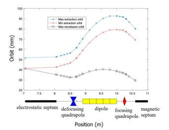
Fig. 6 Simulated extraction orbit
