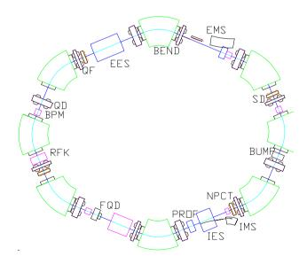
**Fig. 2** Magnetic lattice structure of the SAPT synchrotron (QF: focusing quadrupole, QD: defocusing quadrupole, FQD: fast defocusing quadrupole, SD: defocusing sextupole, RFK: radio frequency kicker, BEND: dipole magnet, BUMP: bump magnet, BPM: beam position monitor, PROF: profile monitor, NPCT: current transformer, IES: injection electrostatic septum, IMS: injection magnetic septum, EES: extraction electrostatic septum, EMS: extraction magnetic septum)
