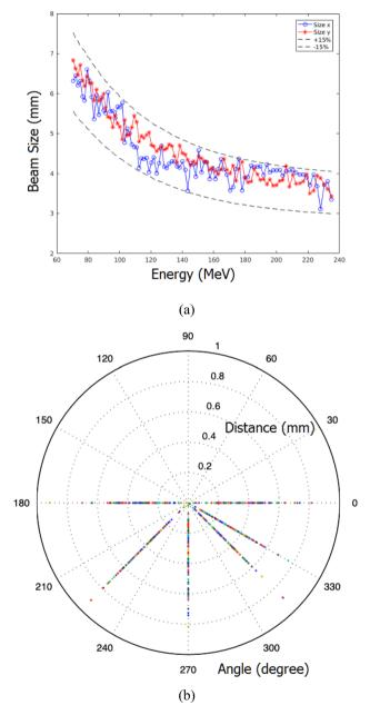
Fig. 10 (Color online) (a) Beam sizes at  $270^{\circ}$  and (b) beam position errors at different angles and different energies
