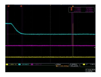
Fig. 9 (Color online) Cutoff time after received signal
